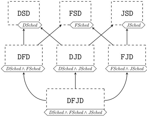
Figure 4: Example of the three-way conflict resolution between the scheduling features. The dashed boxes are deltas. The partial order  $\prec$  is represented by the arrows and each delta  $x \in D$  is decorated with a propositional logic formula representing  $\gamma(x)$ .
