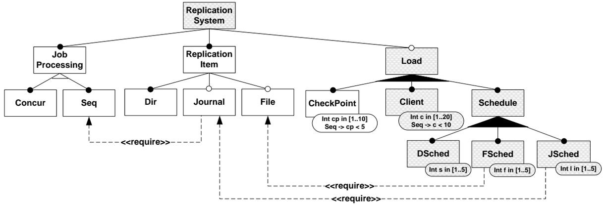
Figure 3: Feature diagram of the replication system
